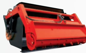
Silo unloader bucket
